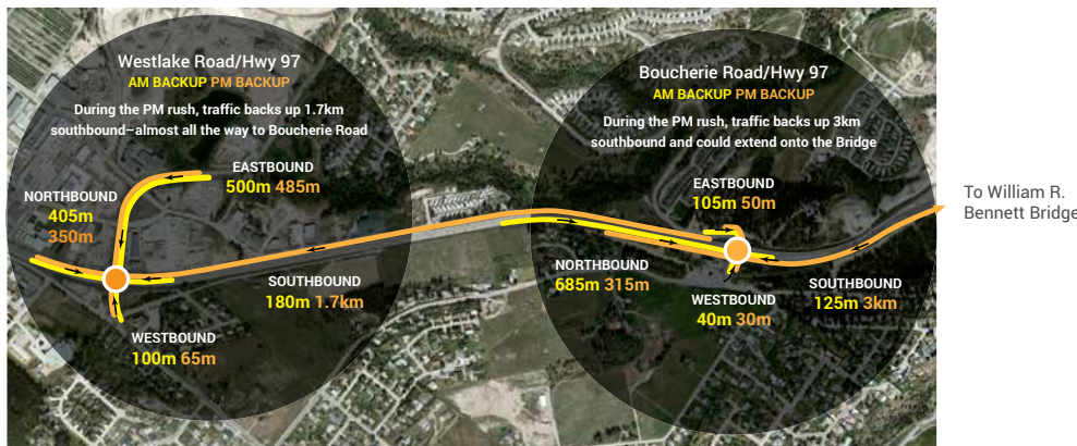
Traffic Backups on Highway 97 During the Morning and Afternoon Peak Hours (Summer 2013)
