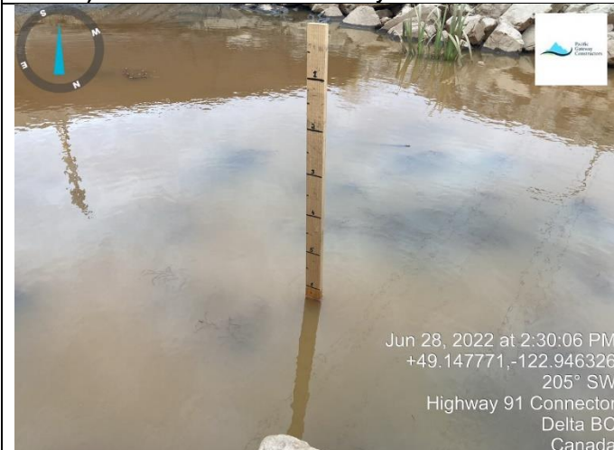
Photo 97: Silda Ditch Upstream showing tidal influence (low tide at 14:22) and water conditions variability.
