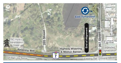
The 287th Street area will function as the east turnaround. The design of the jug-handle turnaround was refined to minimize impacts to private properties. The intersection will include an upgraded leftturn signal from Highway 7 northbound onto 287th Street to address stakeholder concerns about safety.
