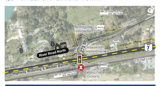
Originally proposed as the west turnaround, 272nd Street and River Road North was reconfigured as a T-intersection to limit property impacts and address steep slope challenges. The West turnaround will now be River Road South loop. This area features residential properties including heritage properties, small businesses, and the Canada Post office.
