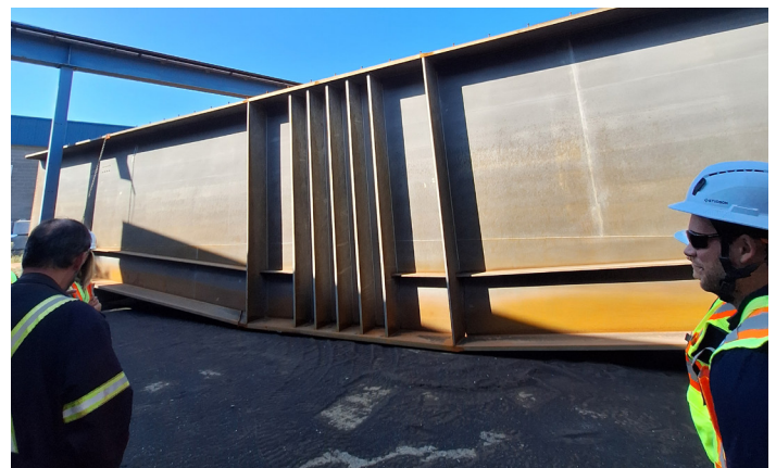
A newly fabricated bridge girder segment (September 2025)
