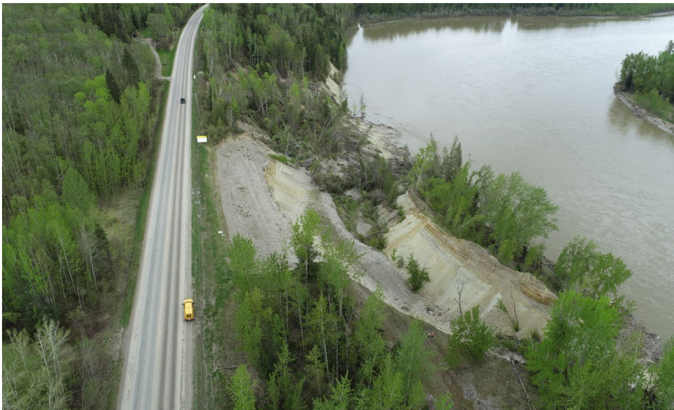
Aerial view of the North Fraser Slide, one of two active slides affecting Blackwater Road.
