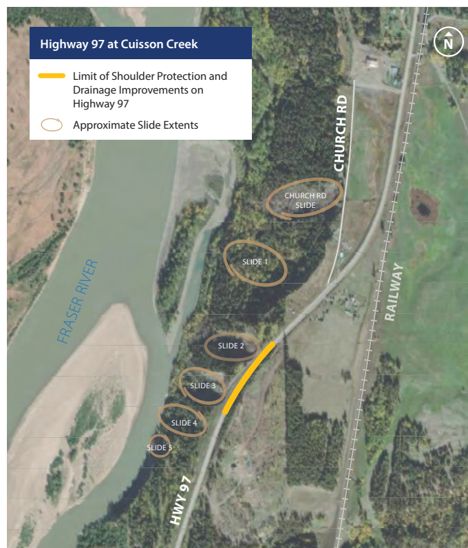
Drainage and shoulder protection improvements on Highway 97 at Cuisson Creek.
