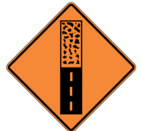
"Pavement ends ahead"
