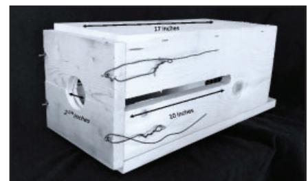
Marten box modified with fisher exclusion plate. The exclusion plate splits in middle and is held in place with wire to allow of extraction of an animal.
