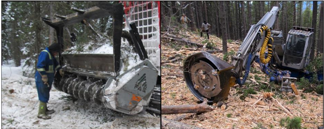
Figure 4: Examples of a drum shaft masticator (left) and disk shaft masticators (right). Images from Hvenegaard and Hsieh (2014) and Steve Hvenegaard. (Used with permission).
