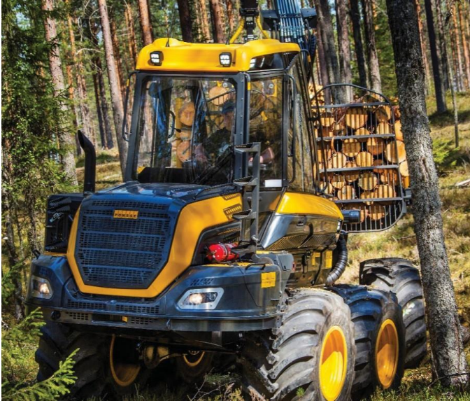
Figure 18. Forwarder removing timber from a partial cut stand. The removal of codominant stems reduces canopy bulk density.
