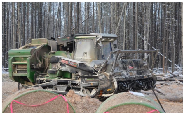
Figure 1. The Gyro-Trac bioenergy baling system (BBS).
