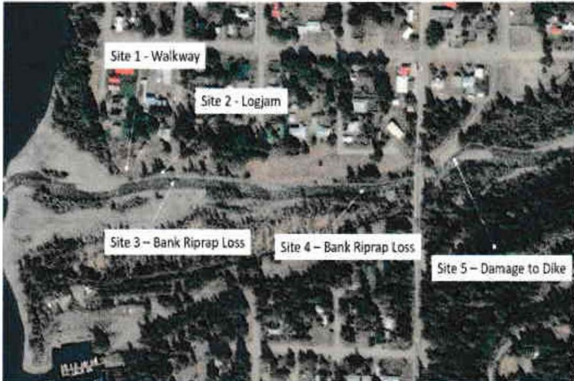
Figure 1: Overview of City of Riverbend- Site Location Map Damaged Sites by flood
