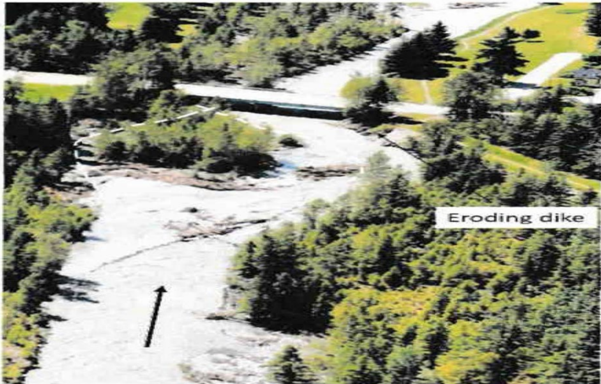
Figure 8b: Site 5 View of mid-channel gravel bar and trees upstream of bridge, June 3, 2020
