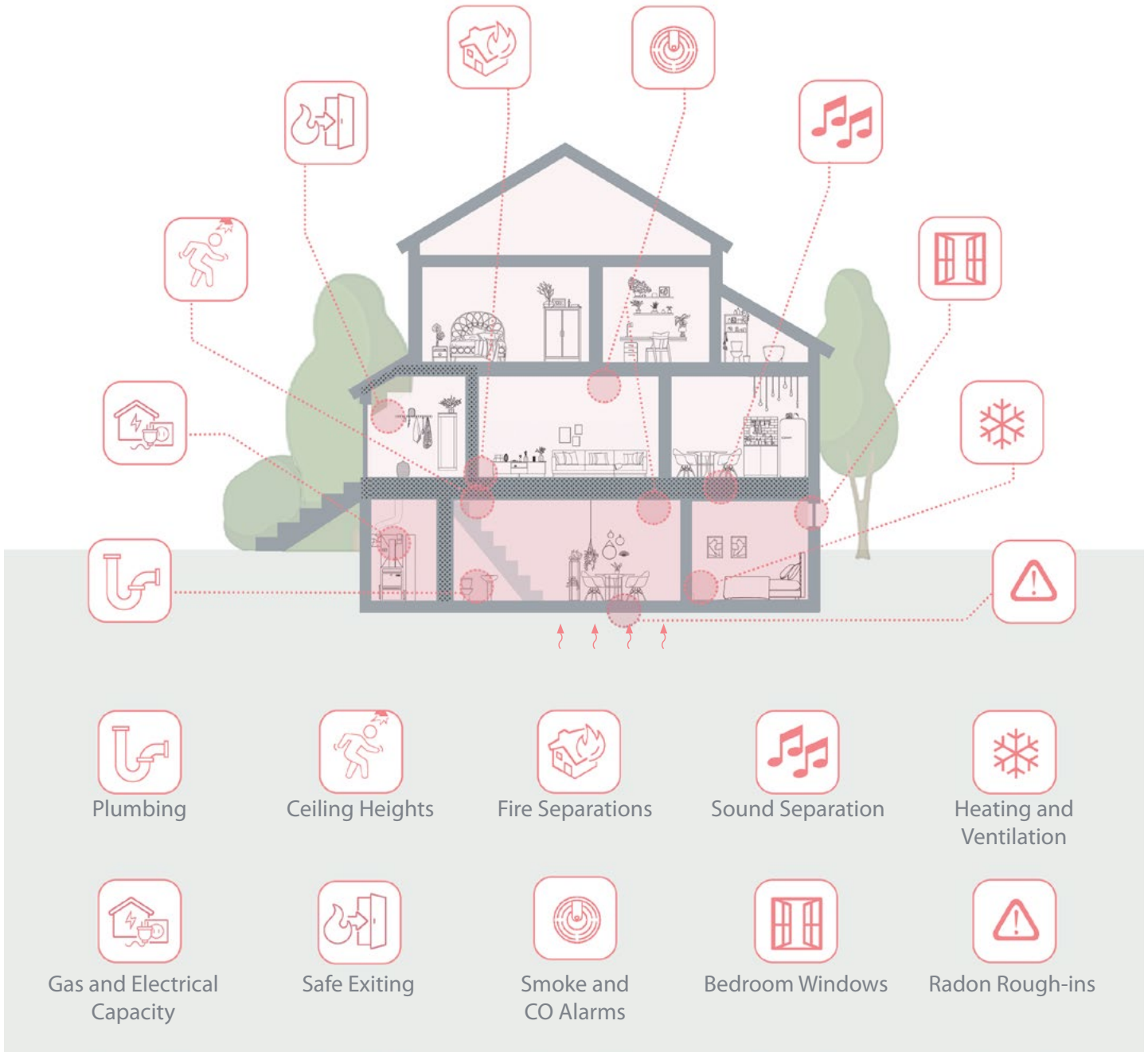
Key Building Code requirements for secondary suites
