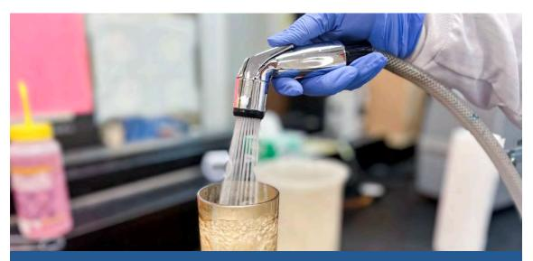
A Laboratory Technologist from the BC Centre for Disease Control Public Health Laboratory is processing drinking water using the membrane filtration technique. This is a provincially approved testing method for drinking water microbiological analysis. Quality assurance practices, such as aseptic technique, buffer washes, and other quality control measures are required to ensure test result reliability. *Photo credit: BC Centre for Disease Control Public Health Laboratory.*
