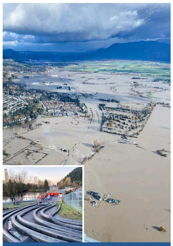
(Top) Flooding in Abbotsford—Sumas Prairie, 2021. (Left) Discharge hosing connected to pumps to draw flood water from the Sumas Canal over the dike at the Barrowtown pump station and into the Fraser River, 2021. Photo credits: City of Abbotsford.
