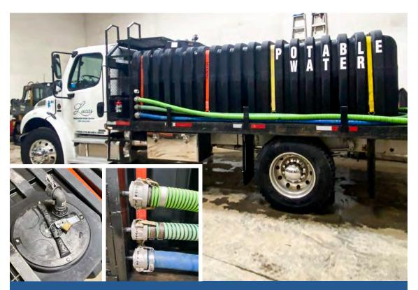
(Above) Northern Health inspecting a bulk water hauler operating out of Charlie Lake (Peace River Regional District). (Left) Lockable access hatch to the potable water tank for monitoring and filling the tank. (Right) Hoses labelled to indicate they are to be used only with potable water. Nozzles are also attached to a connection point to prevent contamination.
