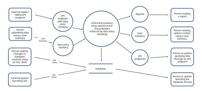
The system might guard against invalid input being entered, then do some processing on the accepted data. It may store the data in a query-able database and/or make the data available to consumers through an API. A dataflow diagram captures all these touchpoints when data needs to be handled in a way that supports Indigenous languages.
