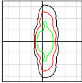
Grid Distance in Units of Mounting Height at 30' Initial Footcandle Values at Grade
