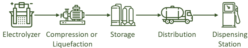
Figure 14: Major Unit Operations of Hydrogen Production via Electrolysis
