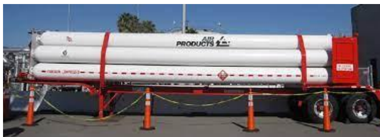
Figure 8: Example hydrogen tube trailer (Source: Air Products)
