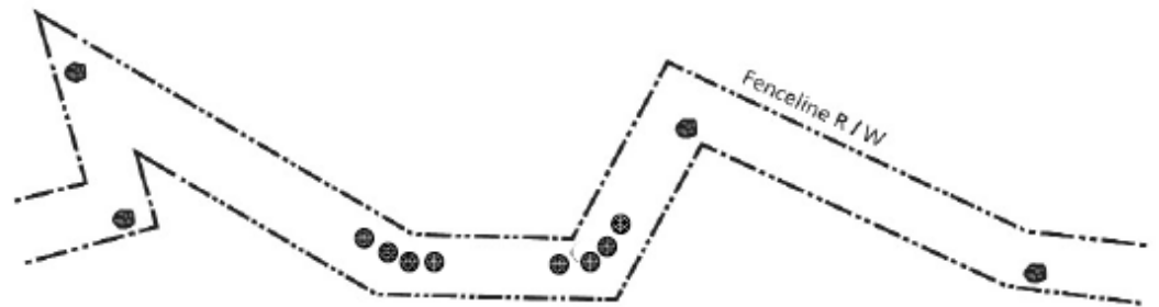
Diagram 1: How to build a straight fence on a crooked right-of-way.
