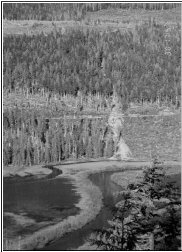
Figure 4. Large seasonal stream flow, relative to 600 mm culvert. Peak flows escaped down the ditch towards top of photo, causing the landslide shown in Figure 5.
