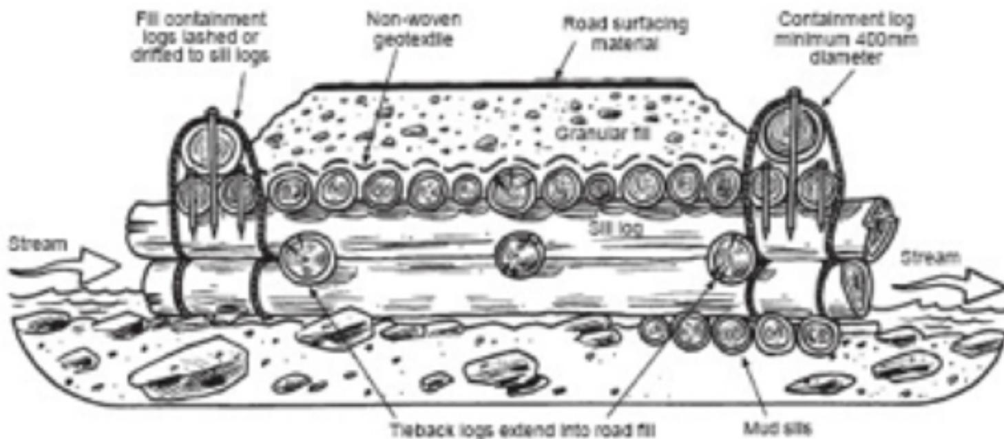
In addition, include provisions that prevent road fill materials from encroaching on the design peak flow discharge flood level. For fills up to 1m thickness, use the sill logs-provided they are long enough-for this purpose. For higher fills, incorporate other site-specific measures into the design.
