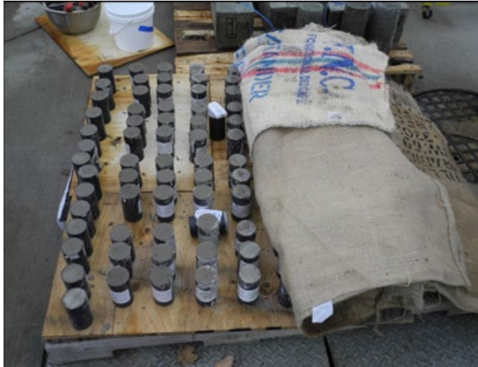
Figure 12: Example of damp burlap sacks being used to keep test specimens cool and moist. Periodically re-wetting the mixture placed in the bridge as well as the test specimens is often required.
