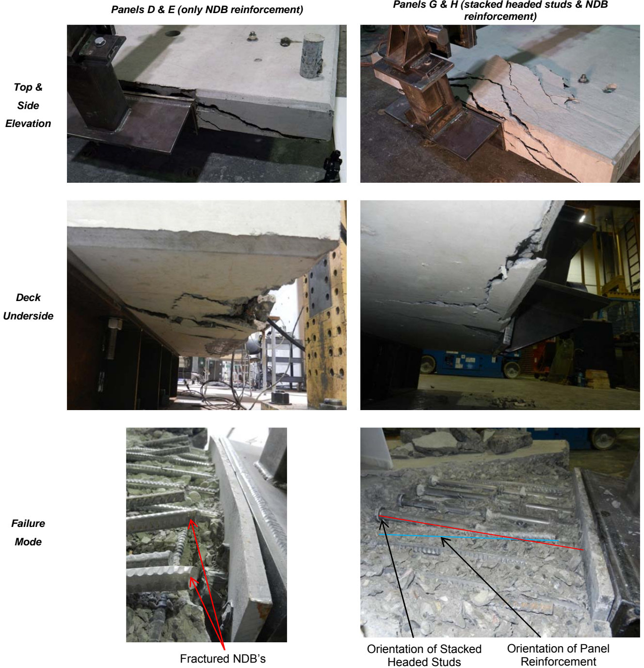
Figure 5-8 Comparison of Original and Modified CL-3 Barrier Connections Failures
