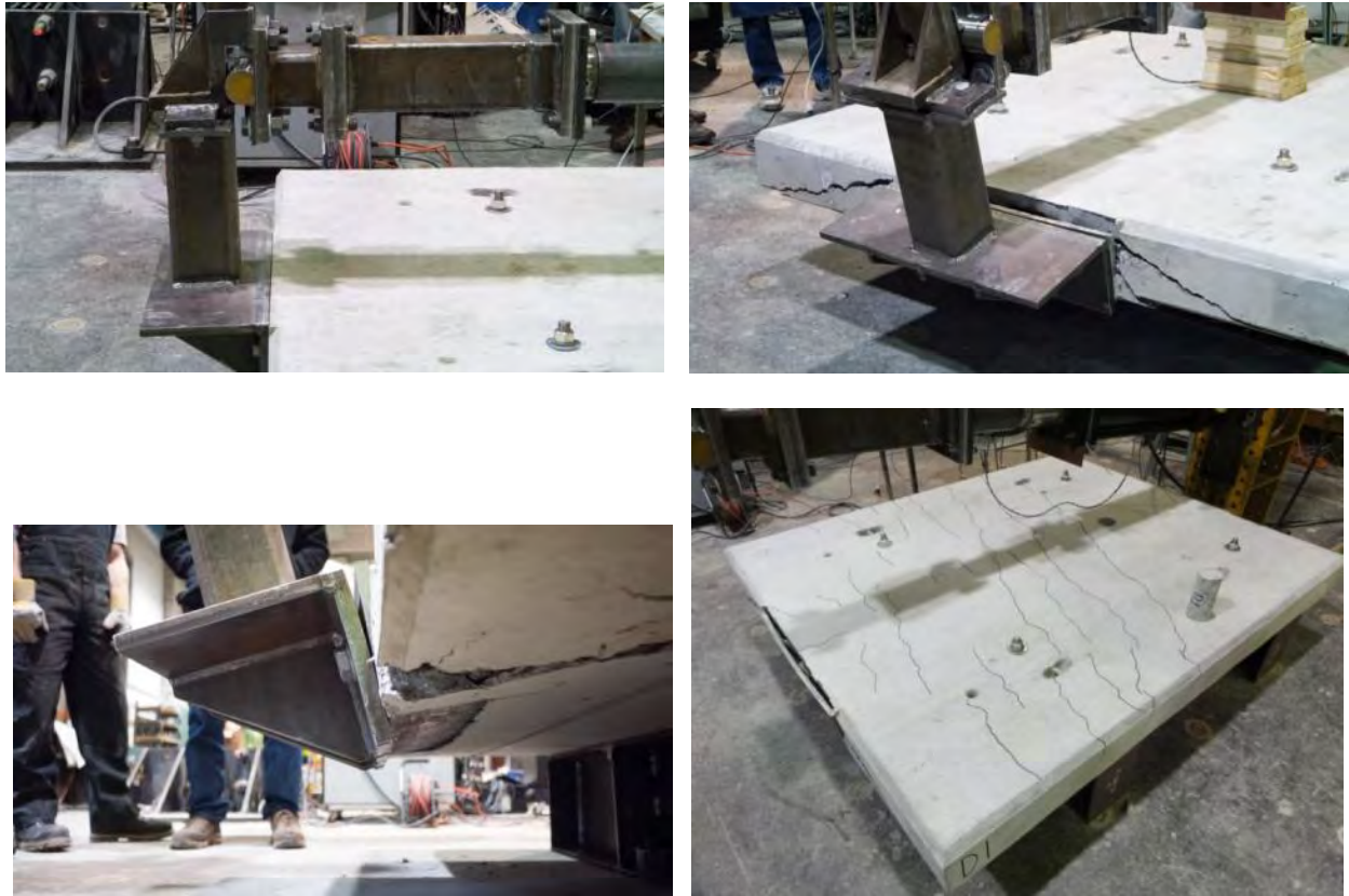
Figure 22: Concrete panel attachment detail failing
