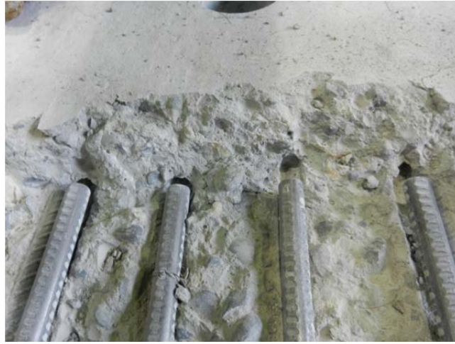
Figure 5-4 Short NDB's Post Failure
