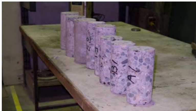
Figure 49: Compression Test Specimen
