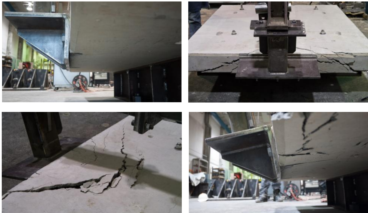
Figure 40: Images from G-1-1, new bolts, slightly longer (1/4")
