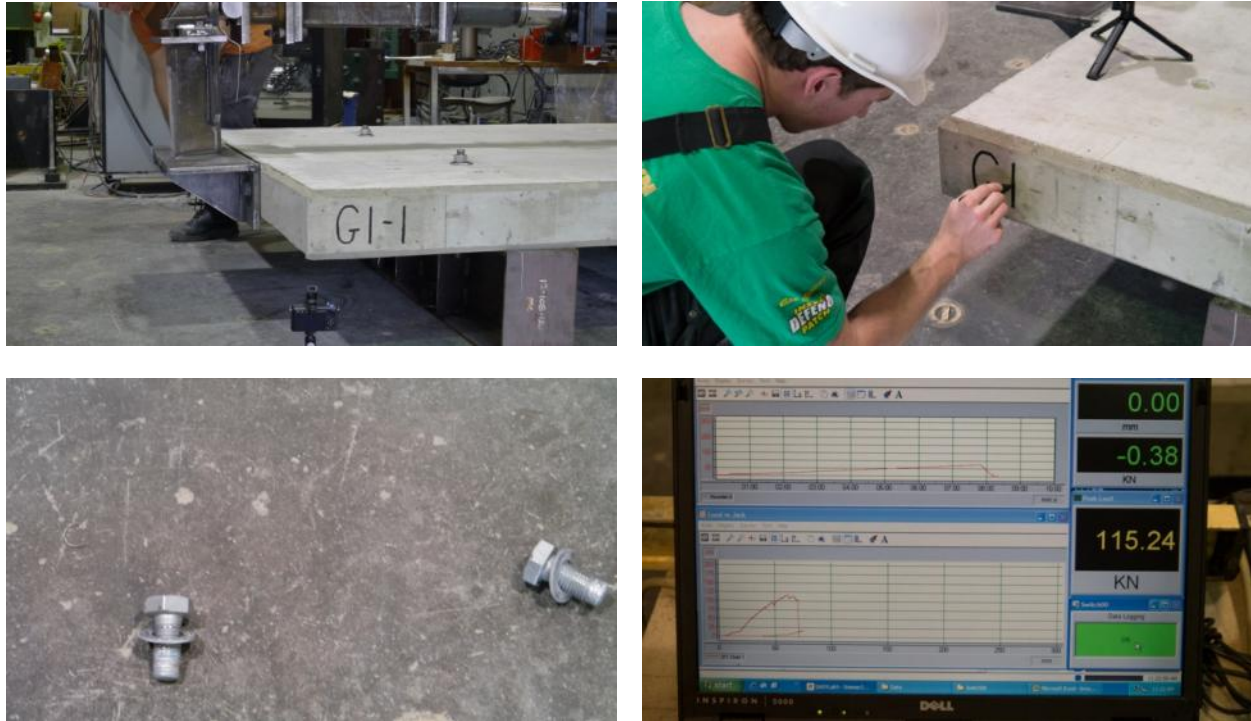
Figure 39: Images from G-1-1, loading to bolts stripping out of sockets
