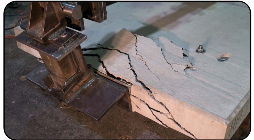
Panels G & H (stacked studs & NDB reinforcement)
