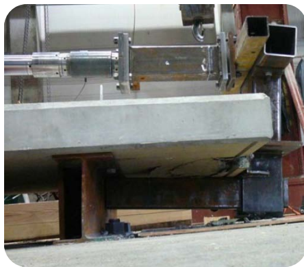
Side Mounted Steel Bracket with Knee-Brace Modification
