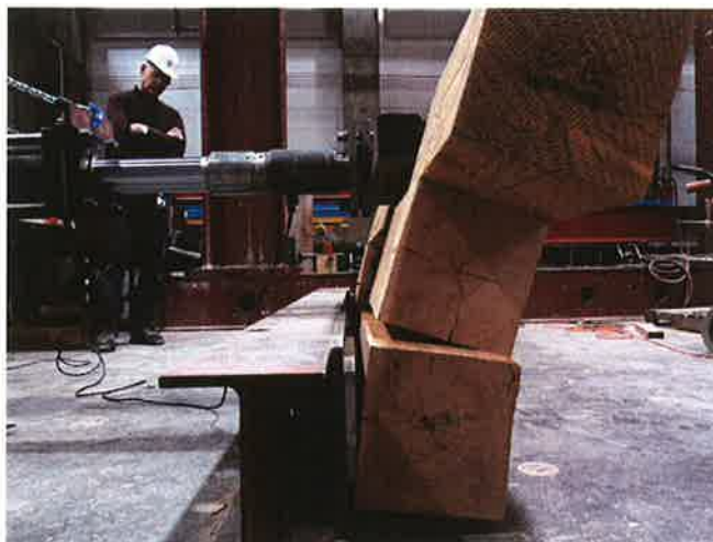
Static testing of timber bridge barrier (courtesy of UBC, 2010)
