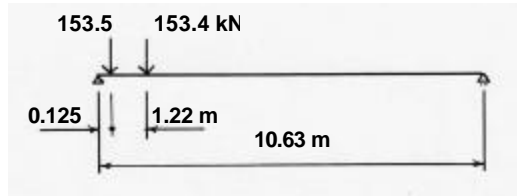
Figure 23 Longitudinal position of Truck A1 on the span of the Harris Creek Bridge
