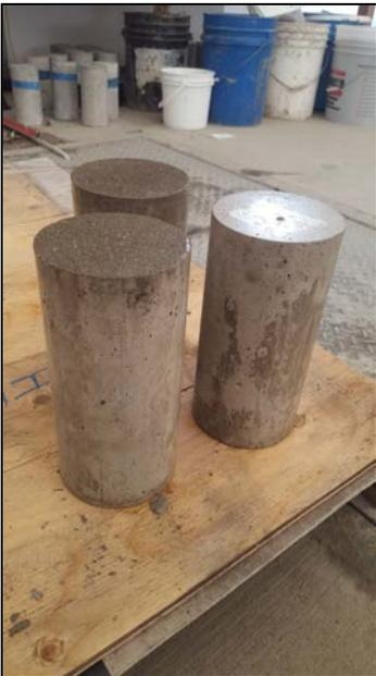
*Figure 1: Ministry Standard 2” test cylinders.*
