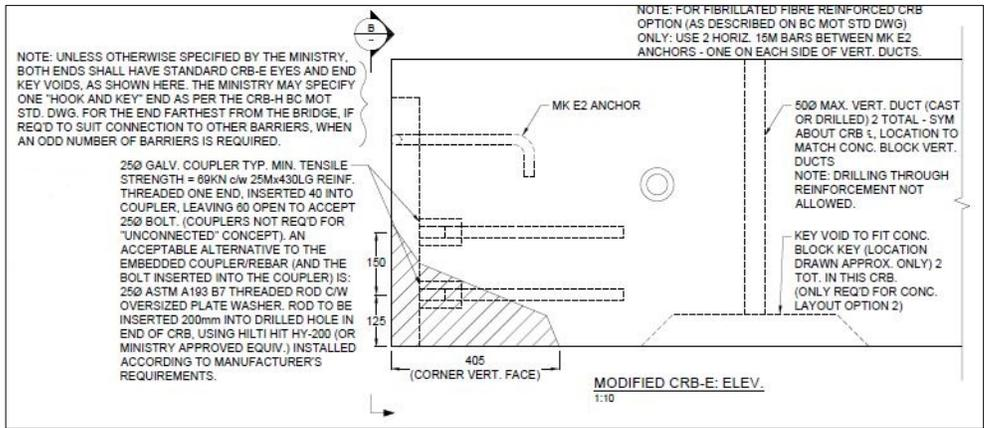
Modified CRB-E (Cast or Drilled Horizontal Threaded Connection)
