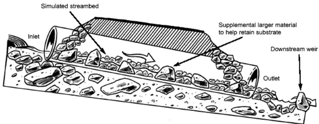
**Figure 1b. Example of a closed-bottom culvert.**
