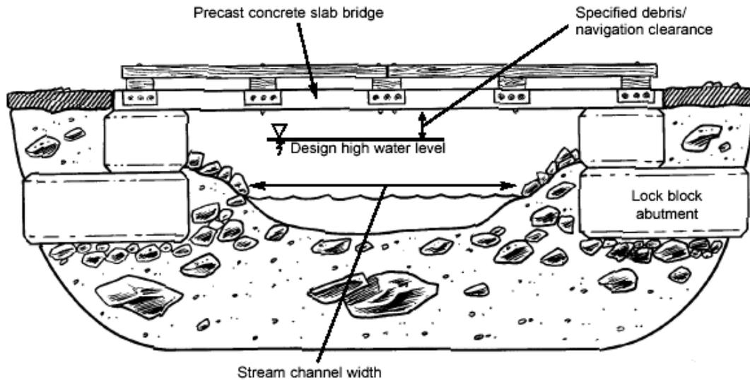
**Figure 1b. Example of a clear-span bridge.** A clear-span bridge is a structure that spans the stream's open water channel and does not involve the construction or installation of any structure between the stream's banks.
