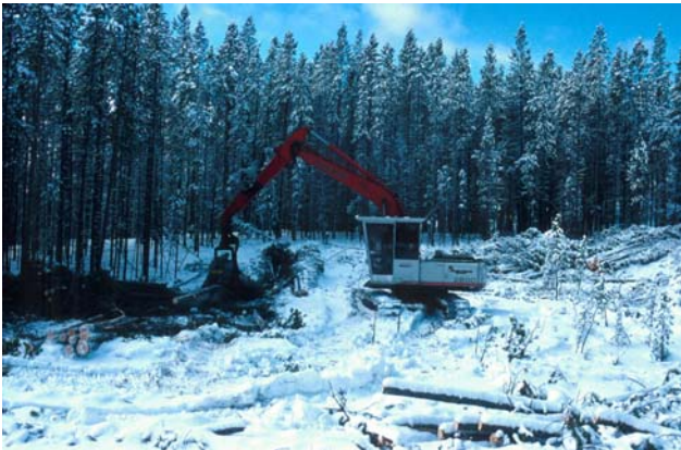
Photo 10. Processing at the stump showing the piling of slash to minimize contact with terrestrial lichens. Photo by Harold Armleder.
