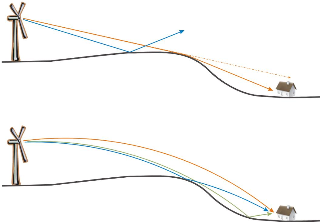
**Figure 2: Model Treatment of Undulating Terrain**
