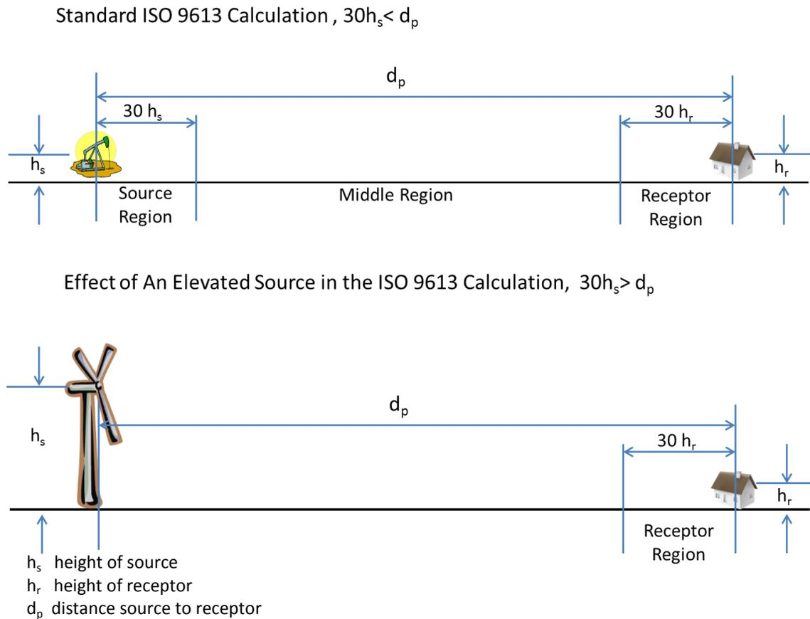
**Figure 1: Illustration of Ground Absorption Calculation**
