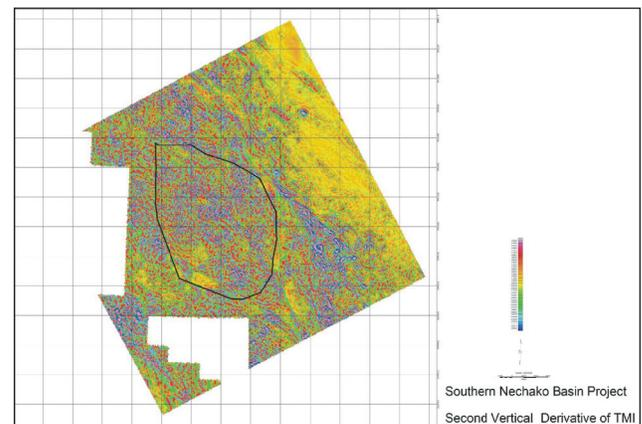
**Figure 4: Second vertical derivative of the TMI map. The location of the gravity survey is outlined on the map for reference.**
