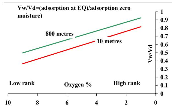
Figure 15. Variation of  $V_w/V_d$  with depth and rank as represented by oxygen content. Data from Joubert, *et al.* (1974).
