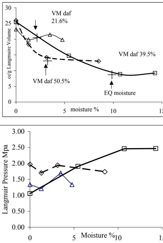
Figure 13. Langmuir Volume and Langmuir Pressure *versus* moisture content below EQ moisture; data from Joubert *et al.* (1974).
