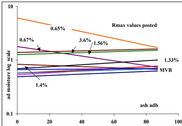
Figure 3. Plots of air-dried moisture *versus* ash for different rank coals.
