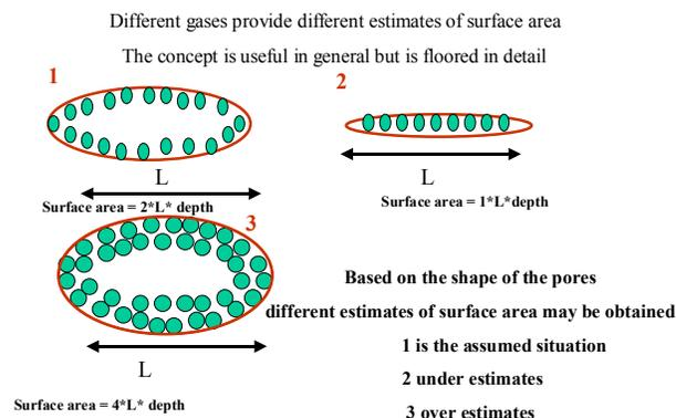
Figure 12. Schematic figure indicating relationship between surface area and adsorption.
