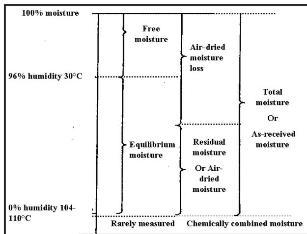
Figure 1. Moisture components in coal.
