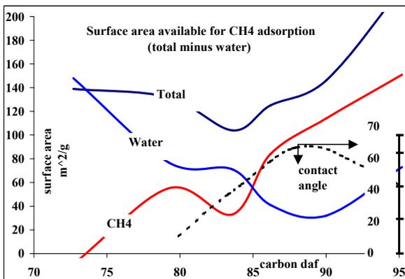
Figure 10. Percent surface area in coal occupied by monolayer adsorbed water; data from Mahajan and Walker (1971).
