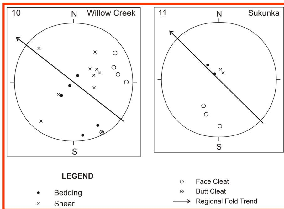
Figure 14. Cleats and fractures in seams at the Willow Creek and Sukunka properties northern Peace River Coal field
