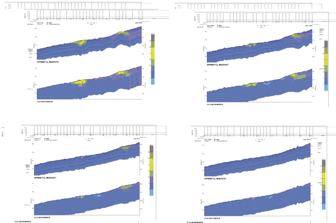
computed using the in-phase and quadrature data at all 5 frequencies.
