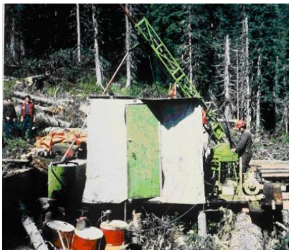
Heliportable diamond drill—large clearing required for crew changes with helicopter.
