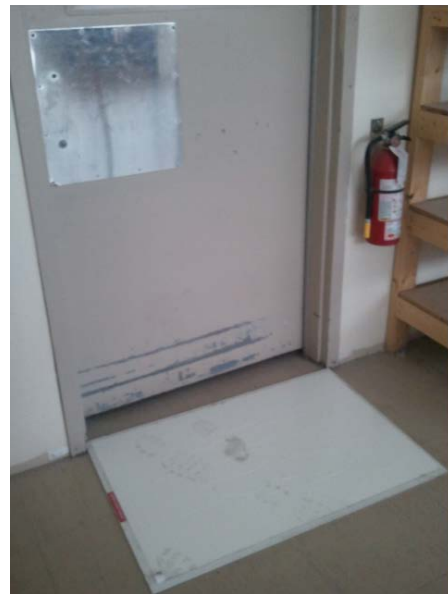
Figure 6: A sticky door mat placed on the inside of the fire assay lab to capture dust from workers' boots as they exit.
