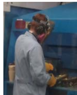
Figure 7: A fire assay worker wearing full PPE while de-slugging samples.
