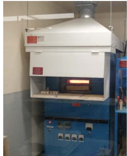
Figure 4: Cupellation furnace equipped with hood space for hot cupels.
