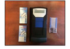
The chip has 10 individual sample tubes. Each tube can only be used once. The tester scans the chip when inserted into the reader and indicates the gas and range for which the chip is designed.
