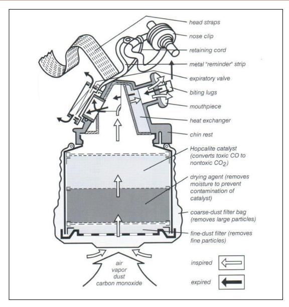
Fig 8-1: How a Self-Rescue functions
