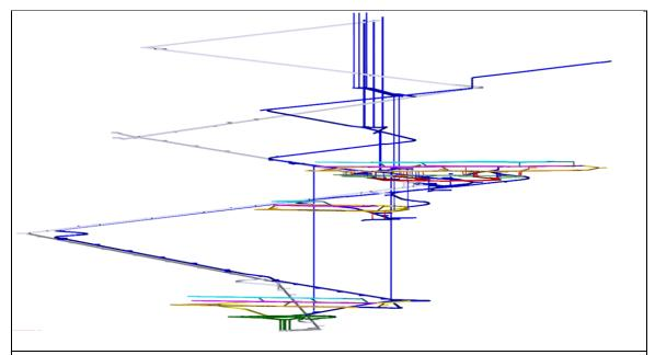
Mines with large vertical dimensions require the use of **sectional views** to obtain a good representation of the mine layout. A section can be thought of as a vertical plan. Mines may have one very long dimension and one short dimension, resulting in the use of two kinds of sections: longitudinal sections along the long dimension and cross-sections across the shorter dimension (the width of the ore body).
