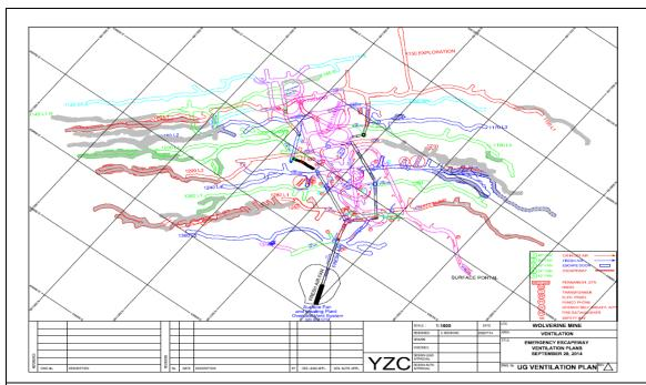
**Plan view mine drawings** provide an overhead view of a mine. Mines will have separate plans drawn for each level in the mine. They are drawn at various scales and the scale will always be noted on the drawing. A legend will be included to indicate the symbols used for fans, ventilation doors, shafts, raises, ore passes and so on. The symbols may vary from mine to mine.
