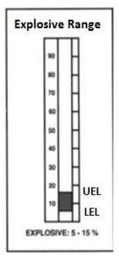
Fig 5.1 Relative density and Explosive range for Methane
