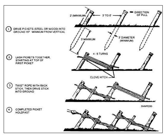
Multiple anchor points may be required to establish a bombproof anchor. Remember the 10:1 safety factor.
