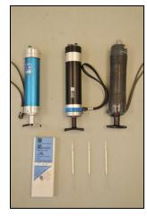
Drager (L) and Gastec (R) colorimetric tubes
