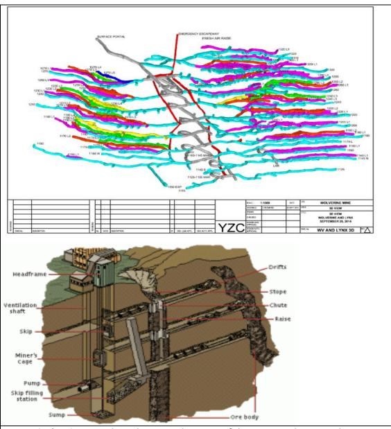
**Isometric drawings** are three-dimensional pictures of the mine workings. It shows what the workings would look like if all the rock surrounding the mine openings was transparent. With the advent of trackless mining methods using inclined and spiral ramps, normal mine drawings become quite difficult to read unless you are familiar with the mine layout, whereas isometric drawings provide a quick overview.
