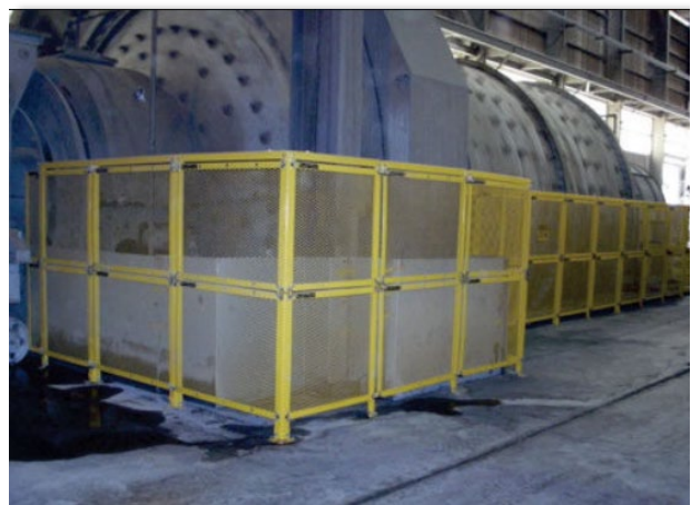
FIGURE 10: DISTANCE GUARD EXAMPLE #2
