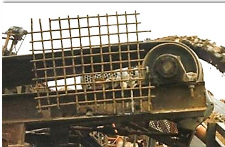
FIGURE 12: EXAMPLE OF A GUARD WITH SNAG/PUNCTURE POINTS
