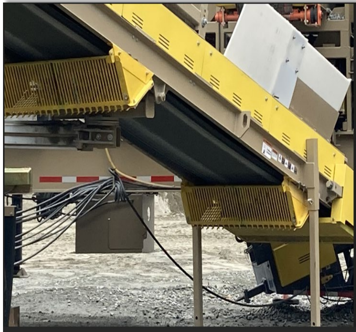
FIGURE 4: EXAMPLES OF RETURN IDLER GUARDING
