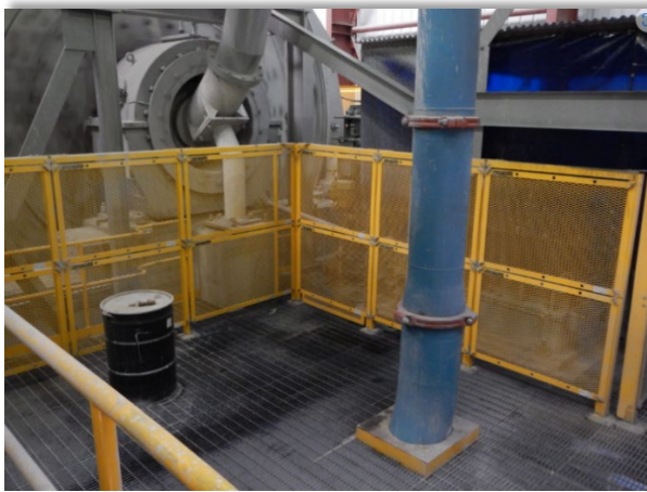
FIGURE 9: DISTANCE GUARD EXAMPLE #1
