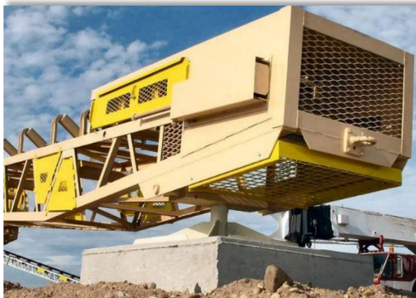
FIGURE 6: GUARD PROTECTING A TAIL PULLEY
