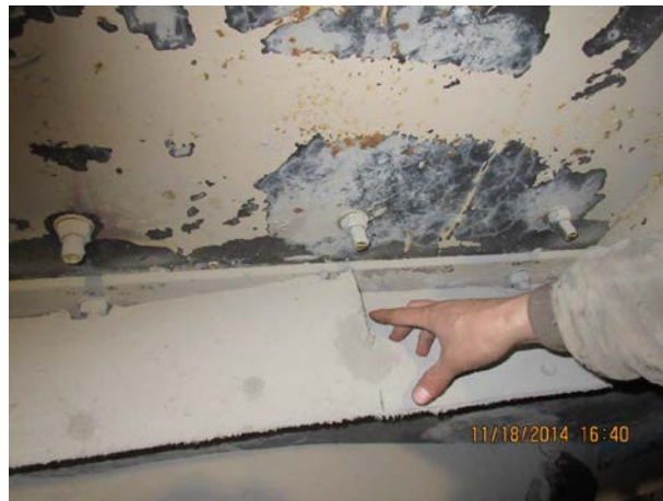
Fine dust that has escaped from skirting on tertiary3 screen deck
