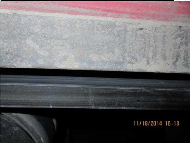
Gap in conveyor skirting #4 conveyor belt
