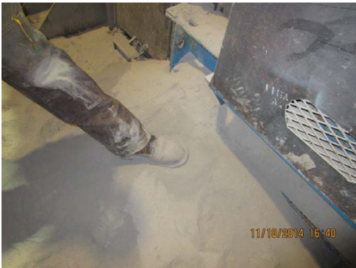
Fine dust that has escaped from skirting on tertiary3 screen deck
