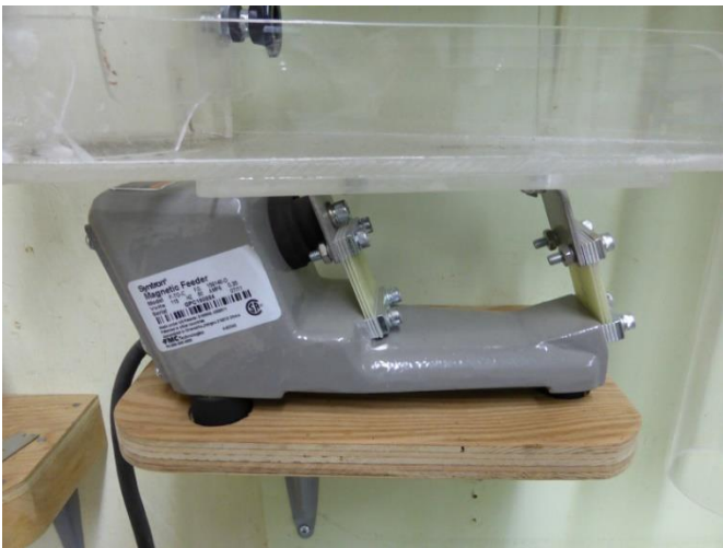
Syntron feeder to regulate the speed of the seed entering the air column.
