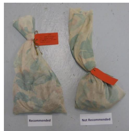
Correct way to tie up sacks.
