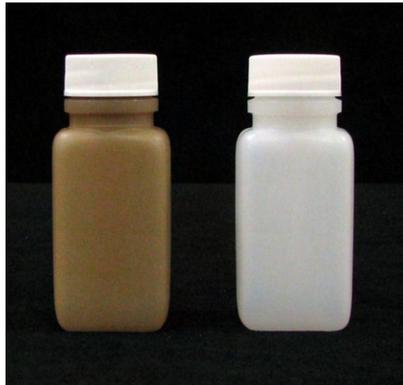
Figure 2. Prototype of the new container, square bottle, 60 ml. Right: HDPE only, Left : HDPE + 7% nano clay which creates the brown color. Photo: MRNF.
