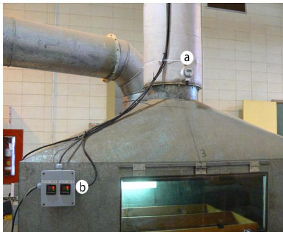
Figure 1. Last section of the Hilleshög seed dryer. a) measurement of the air relative humidity and temperature with a probe connected to b) a control for high (42%) and low (33%) limits of relative humidity. Photo: MRNF.
