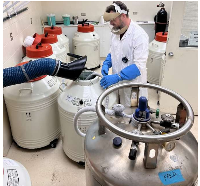
Figure 1: Image of NTSC staff member Matt Brophy filling cryogenic storage tanks with liquid nitrogen
