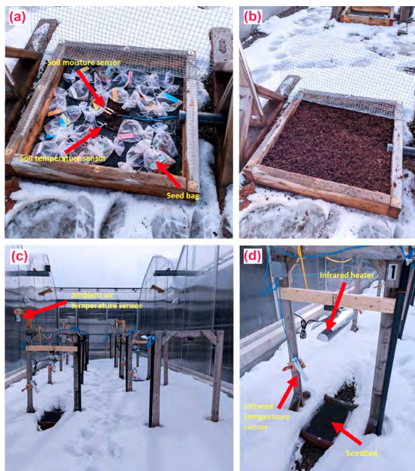
Figure 1. Seed plot layout and design: (a) arrangement of the 24 seed bags (50 seeds per bag \times four seedlots \times six species) within one seedbed and locations of the soil temperature and moisture sensors; (b) the seedbed after the seed bags were covered with peat moss; (c) the entire site where the eight plots were set up in two rows of four (the closest plot was not used) and the location of one of the ambient air temperature sensors; and (d) location of the seedbed relative to the infrared heater and infrared temperature sensor.
