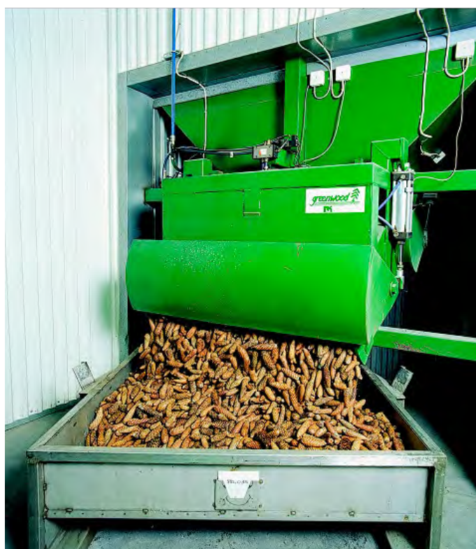
Figure 3. The cone filler is used for getting the right volume of cones into one kiln box. The filler was custom made for our facility when it was established during the 1980s.
