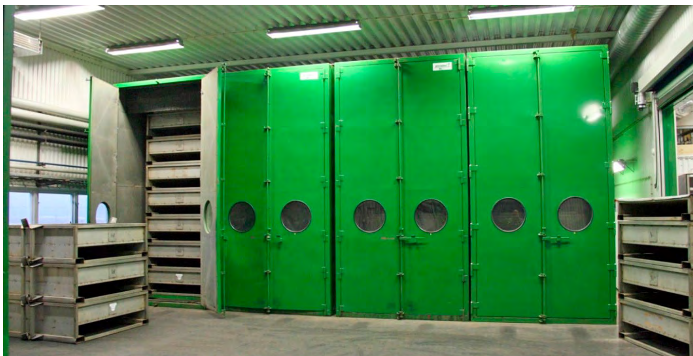
Figure 4. Our four kiln ovens. Each kiln can be monitored individually to track the temperature during the drying program.
