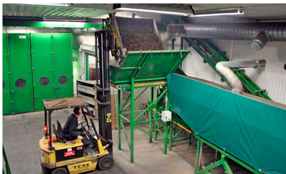
Figure 5. Time to get the seed out of the cones using a rotating drum. Cones are first fork-lifted up and dumped into the hopper.
