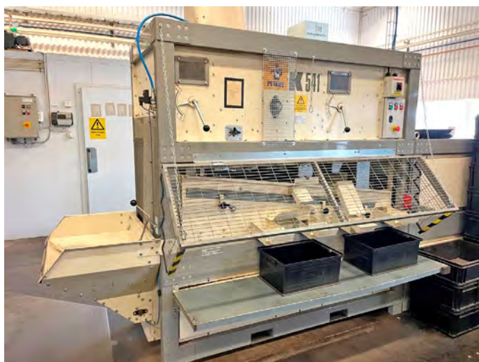
Figure 8. To achieve as high-quality seed as possible the final step performed is using the seed cleaner (Petkus K541) three times for each seed batch.
