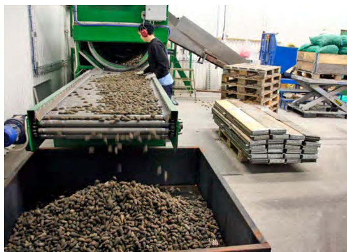
Figure 2. First step is mechanical pre-screening and manual sorting of cones from debris. Photo: Finnvid Prescher.
