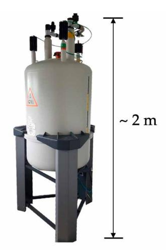
Figure 1. MRI scanner with 11.74 T magnetic field strength. Sample is lowered to the center of the cylinder from the top using an airlift. Magnetic field is created by a current running in a loop of superconducting material cooled using liquid helium (4 Kelvin, -269°C). Helium evaporation is minimized with nitrogen (77 Kelvin, -196°C) surrounding the helium.
