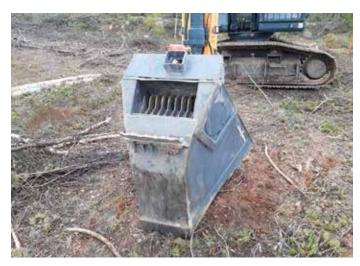
Figure 1. Improved version of the direct seeding bucket (DSB) equipped with a separate scarification blade.
