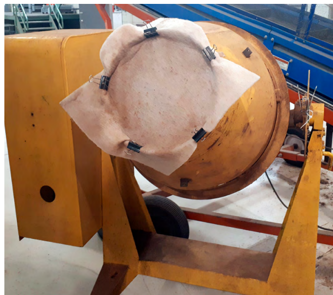
Figure 1. Cement mixer used for dewinging yellow birch seeds. The white cloth limits dust inhalation by staff.
