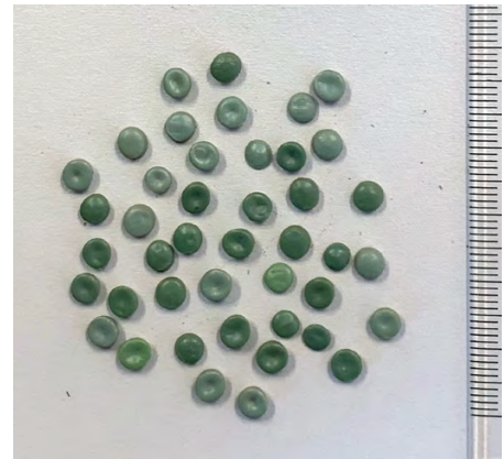
Figure 6. Spherical granules (lens type) made of regenerated recycled high-density polyethylene (reprocess). Each particle has a diameter of about 5 mm.
