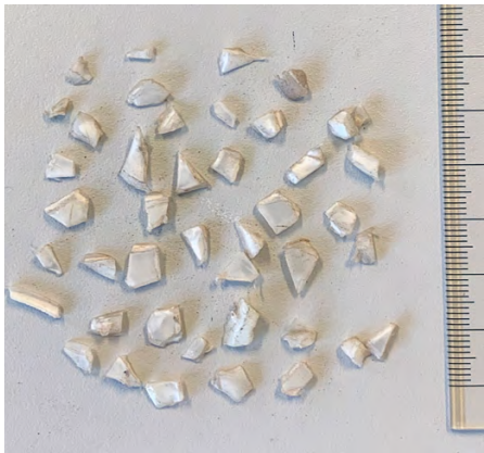
Figure 4. Polypropylene granules (PP regrind). Note the irregular shape.
