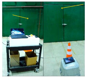
Figure 5. Using endoscopes to observe cone opening on a laptop and tablet.
