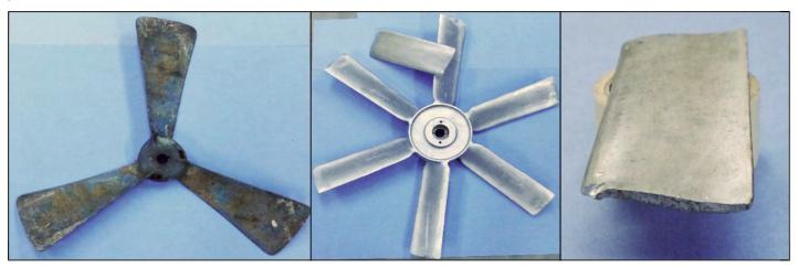
Figure 3. Kiln fans: the old, the new, and the broken blade.
