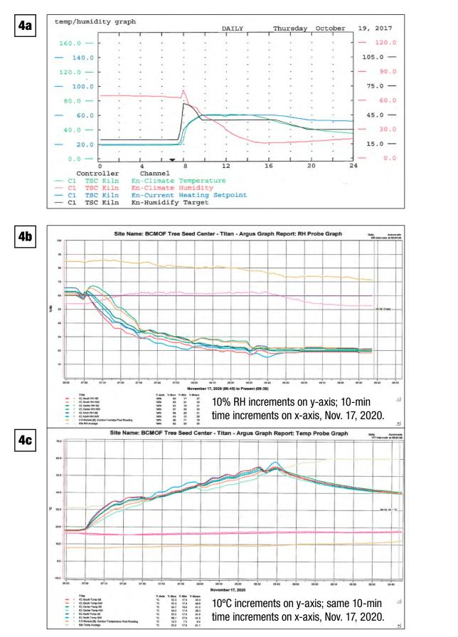
Figure 4. Kiln run graphs from the old (a) and new (b, c) software programs.
