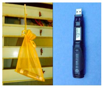
Figure 2. A downloadable temperature and RH% data logger placed inside the kiln.
