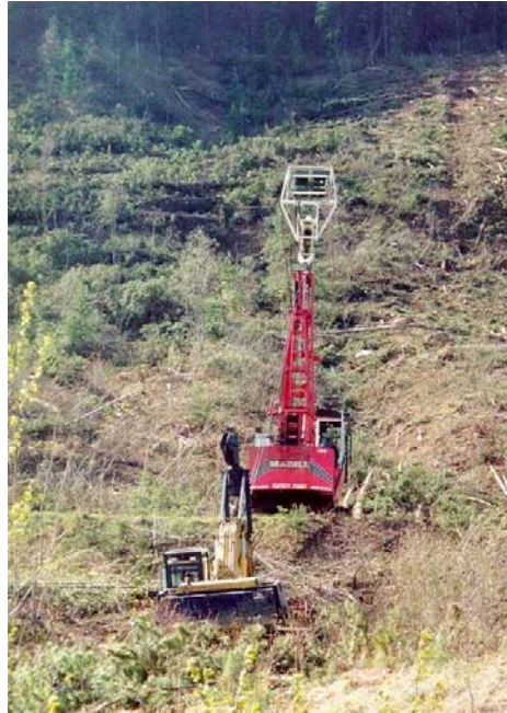
Photo 9: Grapple yarding is used to address steep or sensitive sites.
