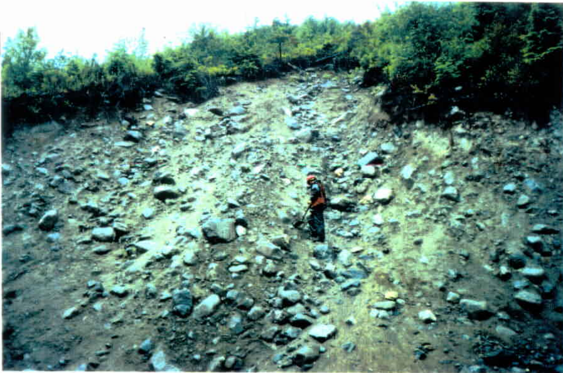
Photo 5: Thick ablation till exposed in roadcuts in Elaho valley (E-600, Site AC37). Material has a much higher proportion of clasts (stones) and less fines than basal till. It is relatively loose and subject to raveling in road cuts. (Photo A. Collett)
