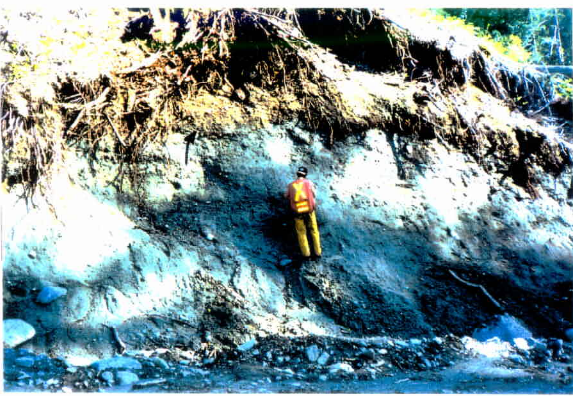
Photo 4: Thick, highly consolidated till with few boulders in road cut at Site ST25. Note sharp contact between weathered (soil) and unweathered till (arrow). This contact is usually the lower limit of the rooting zone, as shown here. (Photo S.Tsang)
